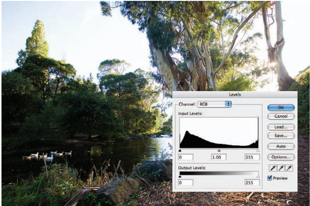
A single exposure in a high-contrast environment could result in a loss of detail in both the shadows and highlights, as can be seen by the tall spikes at Level 0 and Level 255 in the histogram of the image
